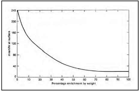
Figure 6-6. Estimated beta dose rate from uranium metal at various enrichment levels (DOE 2001).
