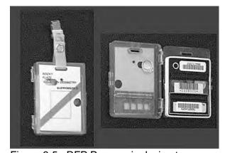
Figure 6-5. RFP Panasonic dosimeter.
