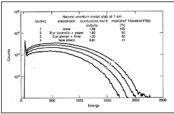
Figure 6-7. Shallow dose rate from natural uranium slab (DOE 2001).
