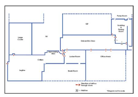
Figure 4. Direction of air flow in the facility observed using ventilation smoke tubes.
