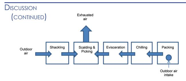
Figure 5. Recommended air flow pattern in a poultry processing facility [Keener 2000].
